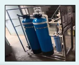
Nanofiltration is a pressure-driven process which is used for treating water by passing it through a semi-permeable membrane. The pore size of the membrane lies between 1-10 nanometers, which is lesser than the pore size of membrane used for ultrafiltration but larger than that of an RO (Reverse Osmosis) process.
